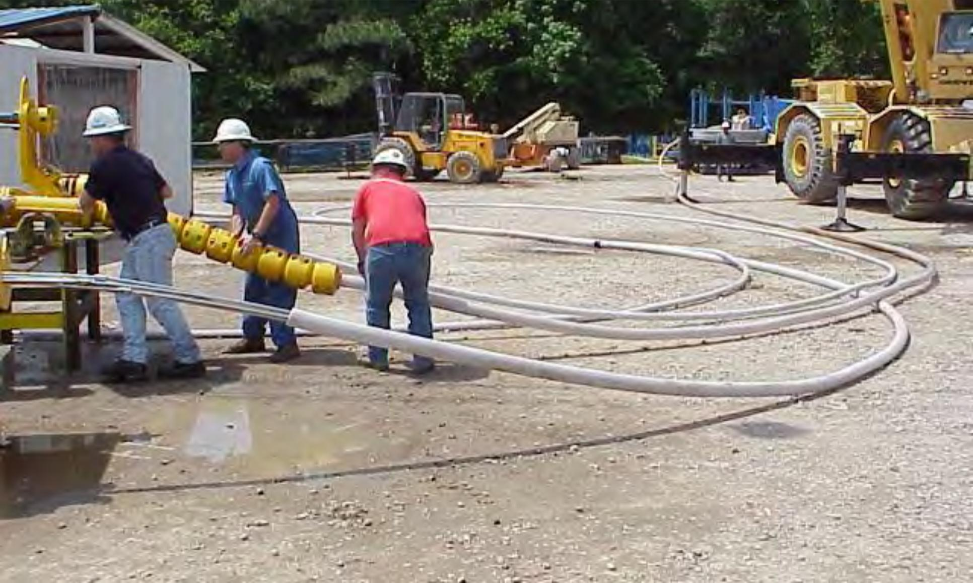
This is not memory, it is flexibility as it sits almost neutrally buoyant on the seafloor waiting to connect to the SUT
